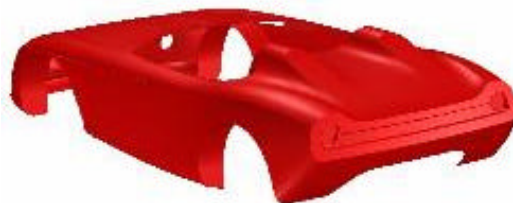
Body surface data used to machine the molds developed by Larry Conger .
