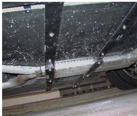
The underbody seat support straps minimize floor panel flexure.
