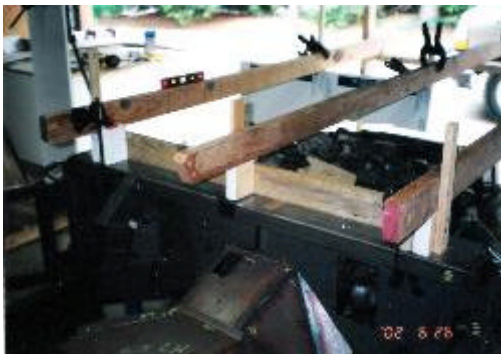
Measuring plane used to accurately determine location of engine components.
