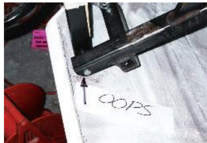
Rear deck temporary positioning fixtures used to position and hold the fiberglass panel in precise alignment before final bonding to the steel support structure.
