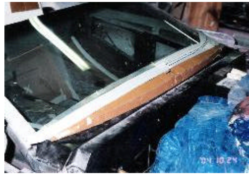
Substrate used to mold the windshield trim panel.
