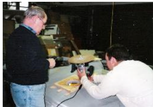
Chuck Carlson (L) and Craig Sandvig routing fuel door hole using fixture.
