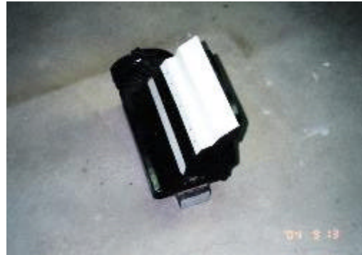
Heater and A/C center distribution chamber.
