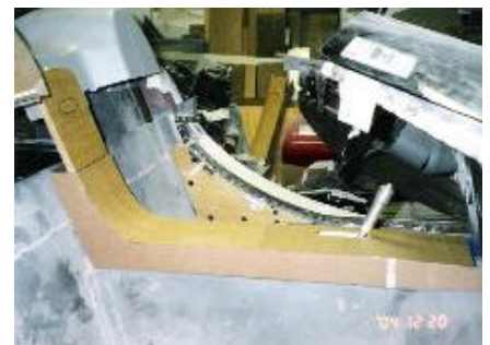
Console mocked up in corrugated paper board.
