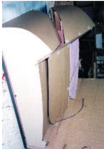
Door cut line study model mocked up in chipboard.
