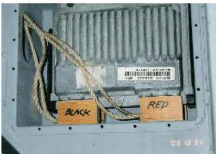
PCM wiring harness mocked up using rope and wood.
