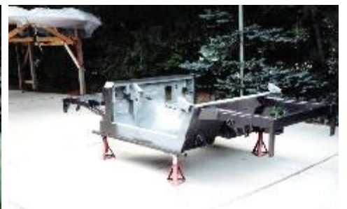
Frame painted and ready for assembly-3/4 rear view.
