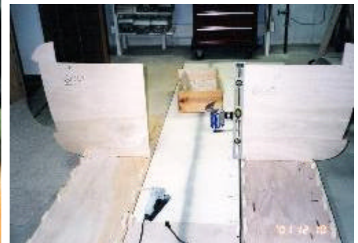
The first two stations being attached to platform for full size foam mock up.
