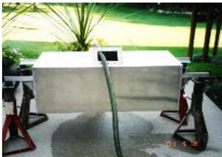
Filling fuel tank with water for leak testing.
