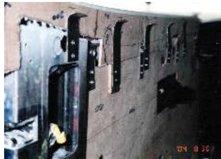
Five steel spring finger tabs hold the upper trim panel against the door flange.
