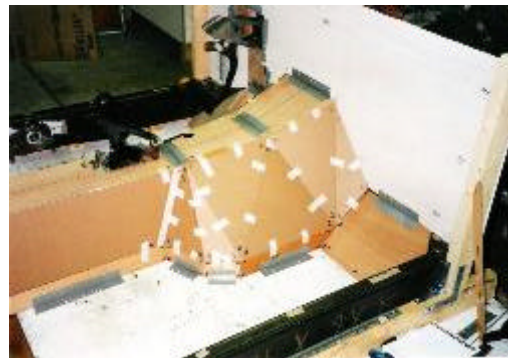
Mock up of transmission tunnel
