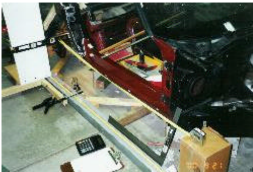
"Bridge" used to measure hundreds of points on the donor vehicle.
