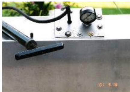
Leak test set up for fuel tank using air pressure on top of water.
