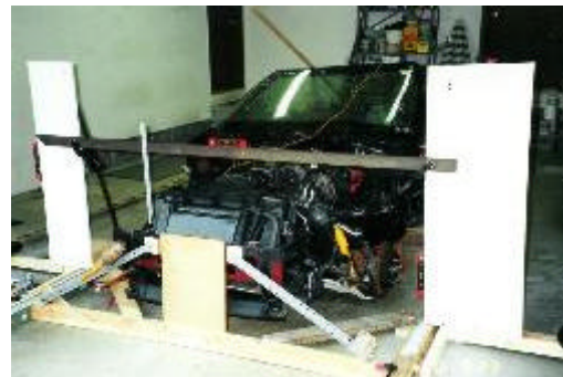
Set up for taking measurements on the donor vehicle.
