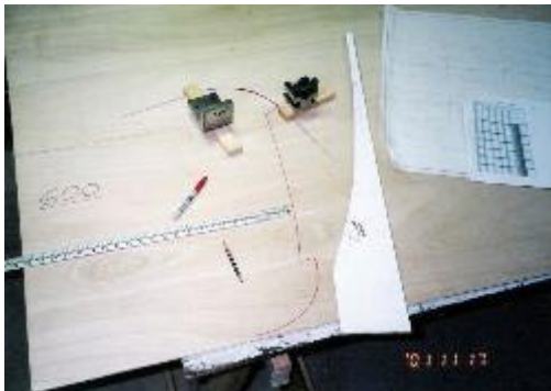
Full size foam mock up Luan plywood station marked for cutting.
