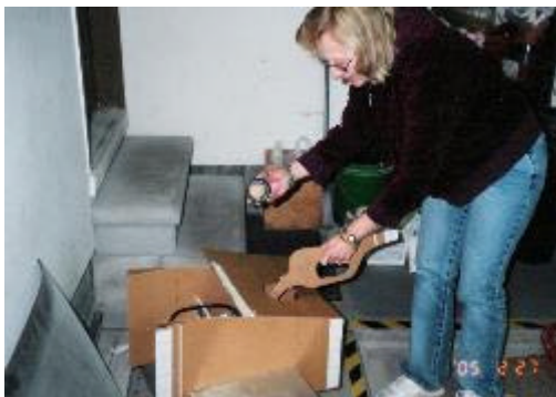
Barbara Dickirson verifying fuel filler door location ergonomics with corrugated paper board mock ups.
