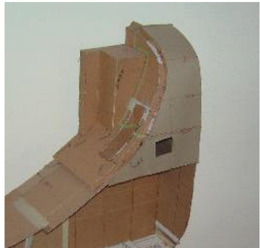
The latch pocket mock up in the rocker panel door sill model.
