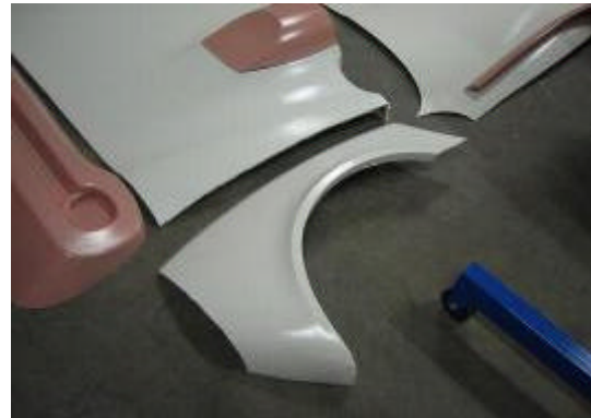
Fiberglass rear deck components after being trimmed.
