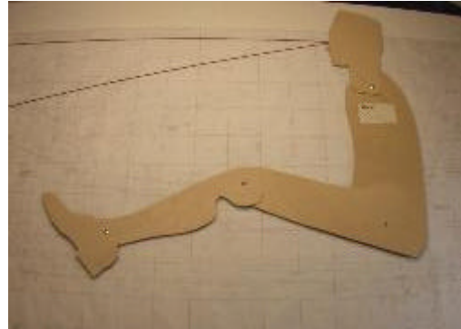
"Biff" the mannequin being used to develop the windshield sight line.
