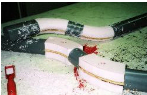
Tail pipes mocked up in plastic tubing, plywood and polystyrene foam.
