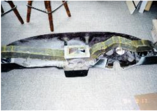
A/C duct fabricated from vinyl ester resin and fiberglass cloth over corrugated paper board.
