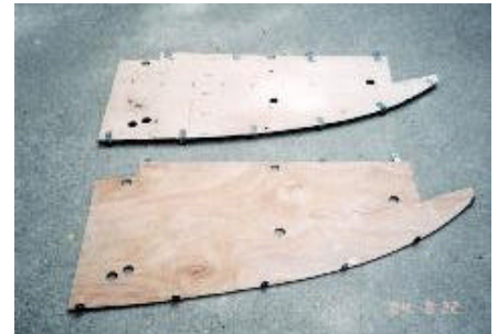
Lauan door trim panel substrates with steel mounting brackets.
