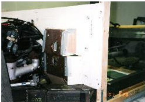
Mock up of dash pockets for brake and steering column mounts.
