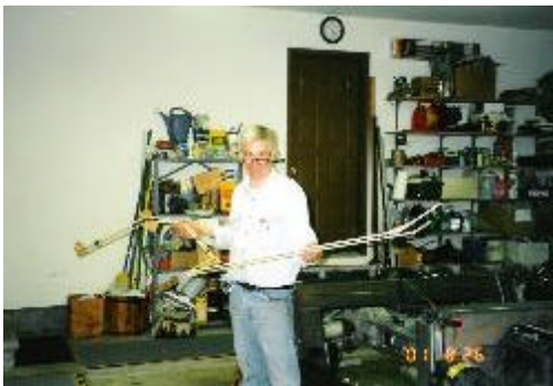
Gene Dickirson with fuel lines mocked up with wood dowel rods.
