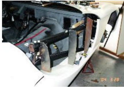
Three steel ribs for attaching door panel to structure.
