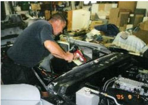
Rick Walsh of Laird's Glass applying adhesive for bonding the windshield to the support structure.
