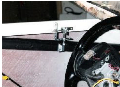
Door panel temporary positioning brackets.
