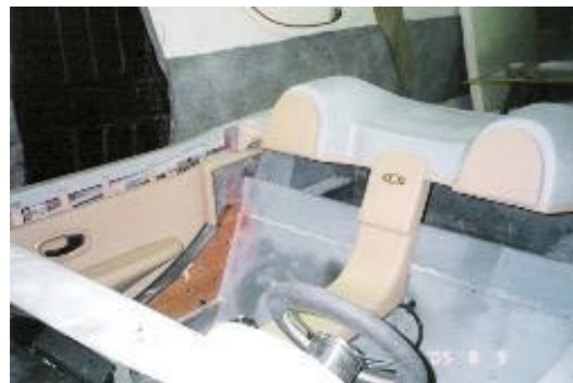
Leather has been applied to most of the interior trim substrates.
