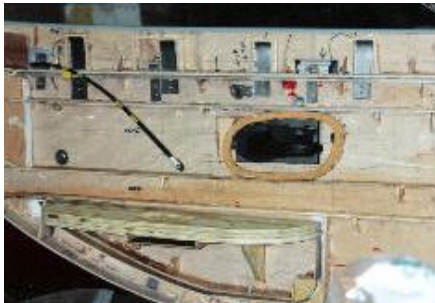
Door trim panel substrate prior to adding polystyrene foam.
