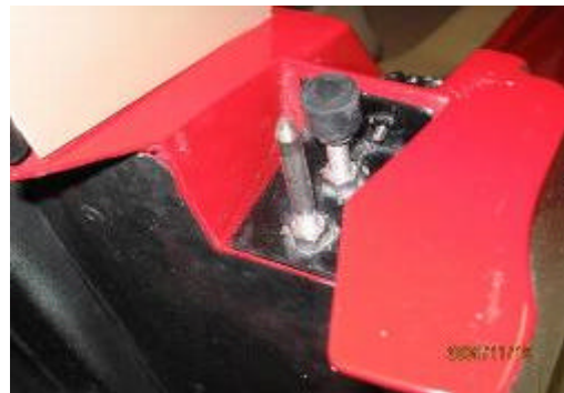
Rear deck alignment pins and bumpers ensure body panels are flush and properly spaced.
