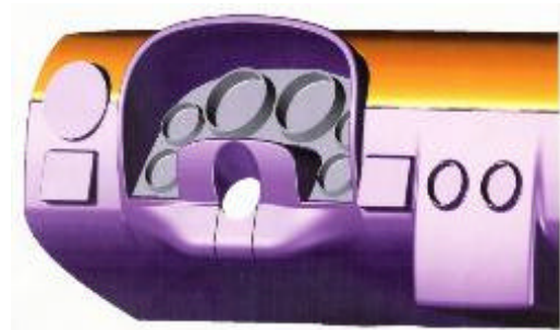
CAD drawing by Larry Conger of instrument panel used to machine the molds.
