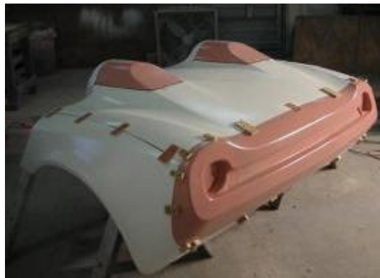
Rear deck components fixtured for bonding.
