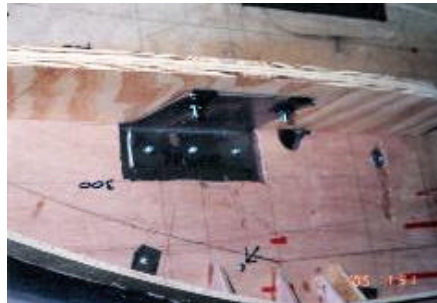
Steel bracket ties door arm rest to door structure.
