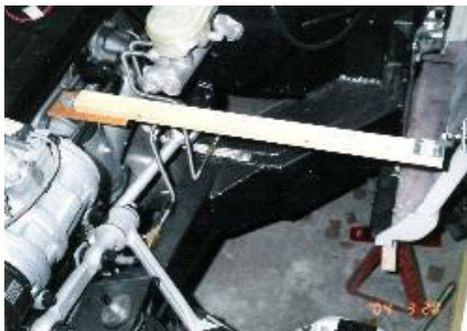
Temporary bracket for locating and holding rocker panel tip during panel bonding process.
