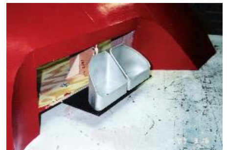
Tail pipe tips mocked up in corrugated paperboard and fiberboard.
