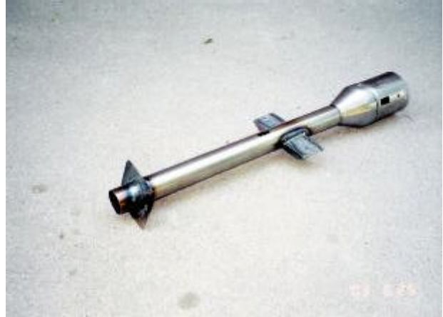
Steering column with mounting brackets welded in place.
