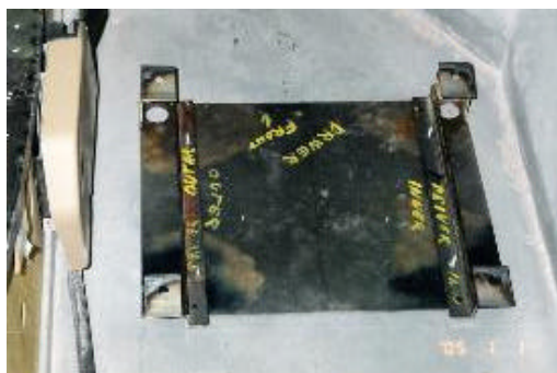
Seat mounting bracket with built in 8.5 degree tilt.
