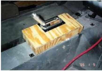
Console mock up in shifter region to develop precise location of opening.
