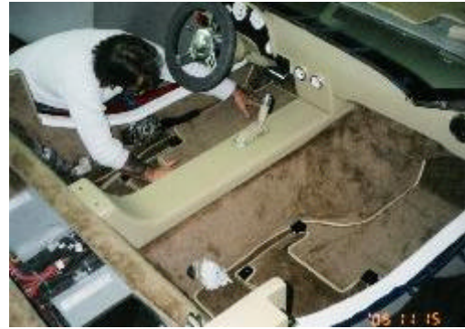
Mark Bowden fitting carpets. Note that the seats can be removed for service without unbonding the surrounding carpet.
