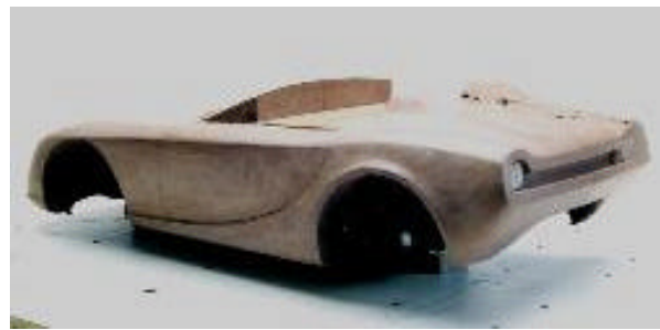
Clay model immediately before it was digitally scanned -3/4 rear view.
