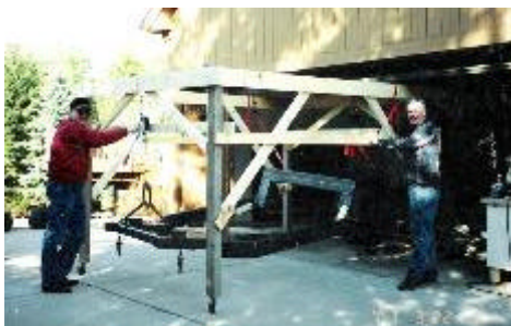
Chuck Carlson (L) and Gene Dickirson with the movable crane used to lift the donor body off the drive train and set the new frame on to the drive train.
