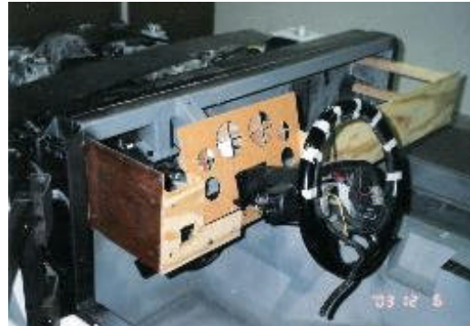
Instrument panel mocked up in plywood to verify switch and gauge locations.
