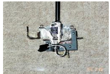
Transmission shifter PRNDL potentiometer and mounting bracket.
