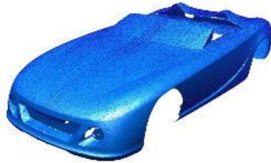
Point Cloud after scanning
