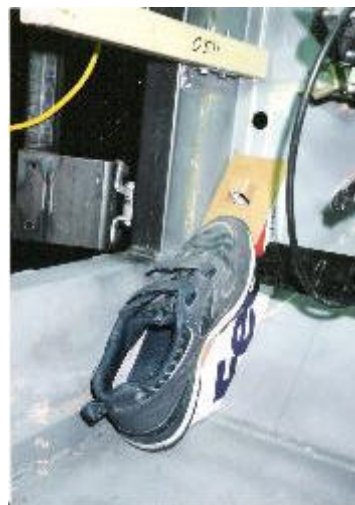
Developing the foot steady rest and head lamp dimmer switch location.
