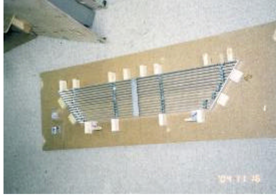
Grill components in weld fixture.
